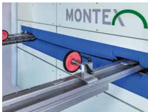
The adjustable and variable slot cover BionicFin
